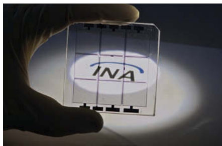
Figure 2: In the "open" position, the view through a micro mirror module is nearly undisturbed, in "closed" position the fill factor is about 95%
