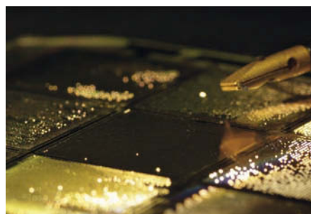
Figure 6: The left-hand image shows micro mirrors reflecting the incident light to the spectator ("mirrors open"). In the right-hand image ("mirrors closed") the mirrors redirect the incident light
